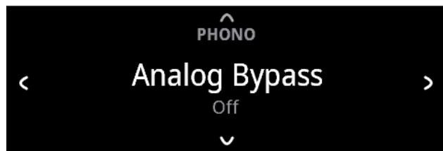
All analog signals remain in the analog domain without analog-to-digital conversions.
