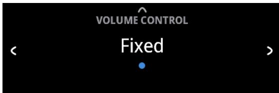
a With "Fixed" level selected and back to "Source Setup" menu selections, use front panel [ $\langle/\rangle$ ] or SR 10's [ $\blacktriangle/\blacktriangleright$ ] buttons to go "Fixed Volume" option. "Fixed Volume" manifests among "Source Setup" options only if "Fixed" is the selected "Volume Control" level.
