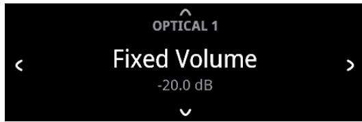
c Use front panel [ $\langle/\rangle$ ] or SR 10's [ $\blacktriangle/\blacktriangleright$ ] buttons to set preferred dB level setting. Then, use front panel [ $\wedge$ ] or SR 10's [ $\blacktriangle$ ] button to save dB level selection and exit Fixed Volume setup mode.
