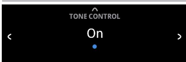
Tone control allows the boosting or reduction of particular audio frequencies. The tone control levels, Bass and Treble, can be turned on or off.
