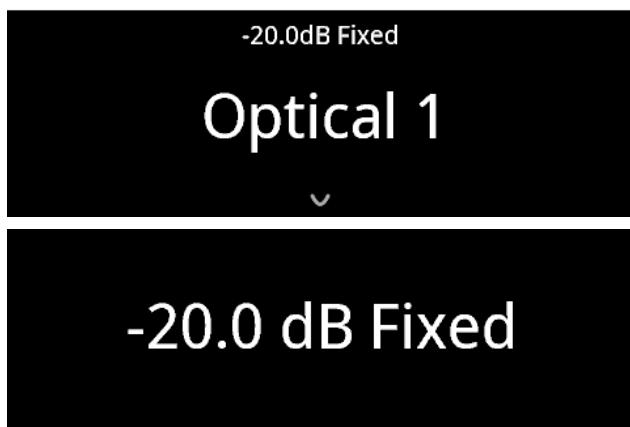
At Fixed volume level setting, front panel display will show "xx.x dB Fixed" as the volume control is adjusted.
