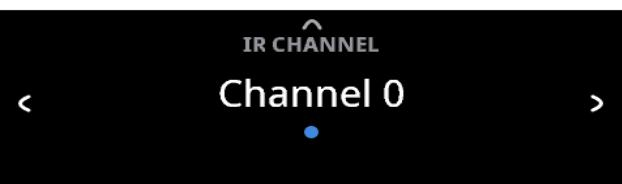
The C 379 has the capability to operate via Alternate IR channel. This is useful if you have two NAD products that can be operated by similar remote control commands. With alternate IR Channel, two different NAD products can be controlled independently in the same zone by setting each one to a different IR channel.
