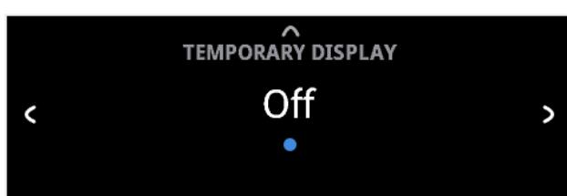
Temporary Display feature enables the display to be turned off temporarily after 30 seconds of non-user interface.
