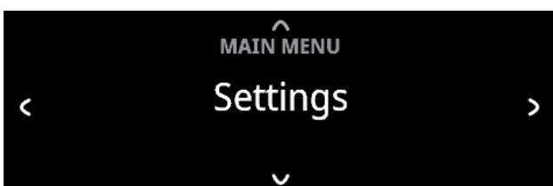
Press front panel [▼] button once for the Main Menu options to appear in the display. Use front panel < or > button to select through the Main Menu options – **Settings**, **Source Setup** and **System Info**.
