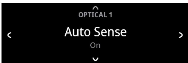
Auto Sense can be setup for each Source. Auto Sense feature enables the designated Source to wake up from standby mode when an active source is detected from the particular Source's input.
