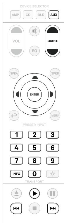
**BluOS PLAYBACK CONTROLS (applicable to NAD products with installed MDC BluOS or MDC2 BluOS D module)** Select **BLS** among the DEVICE SELECTOR buttons to use the following control buttons for BluOS playback.
