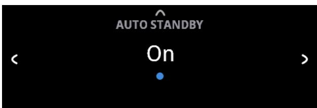
Auto Standby feature is an integral feature of C 379 that conforms to European ecodesign regulations. The C 379 can be setup to automatically go to standby mode if there is no user interface interaction and no active source input within 15 minutes.
